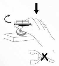
Step 1: Rotate the nut clockwise and install it on the valve
