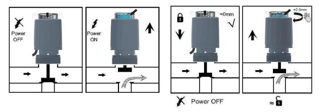
N/C Normally closed (power-on/power-off state)
