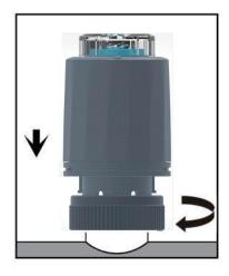
Rotate the nut clockwise and install it on the valve (Note: Do not use pipe pliers, clamp and other tools)
